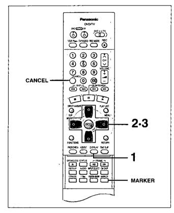
Use on-screen menus to mark, recall, and clear positions. You can also mark positions by pressing [MARKER].
